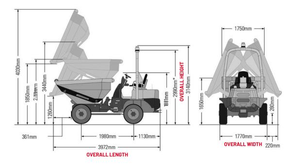
MAX SAFE CARRYING WEIGHT: 3,000KG | LEVELLEDCAPACITY: 1,050L | HEAPEDCAPACITY: 1,760L
